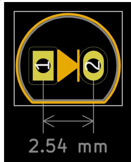
TO-92 diode footprint with standard lead spacing.
