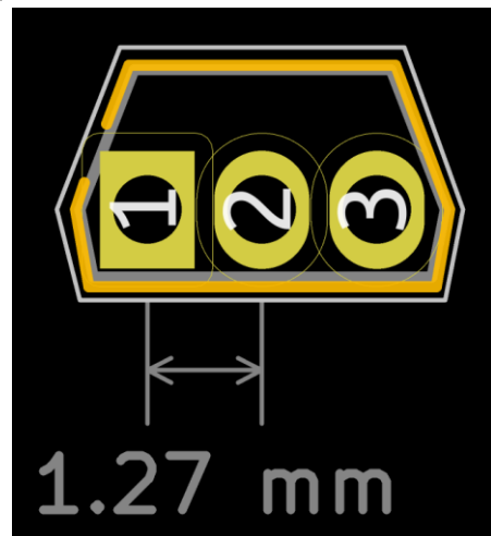
TO-92S footprint with standard lead spacing.
