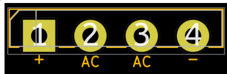
GBL bridge footprint.
