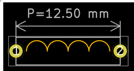
Axial air-core inductor footprint with its pin pitch indicated.
