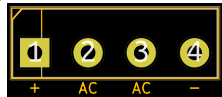
KBL bridge footprint.
